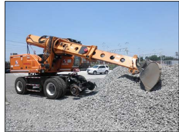
Gradall Hydraulic Excavator with High Rail Gear
